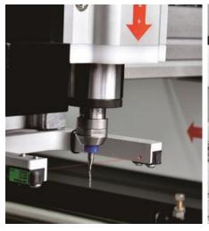
Milling Cutter Detection
