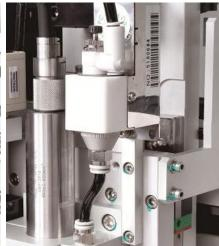
Cutting generates a lot of static, dust will be adsorbed on PCB, annular ion gun structure, gently blowing the ion wind to eliminate static.
